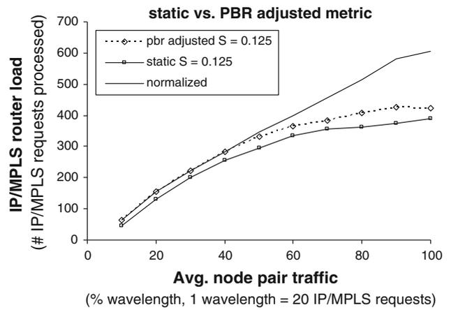
Fig. 7 Static versus PBR adjusted metric; IP/MPLS router loads
