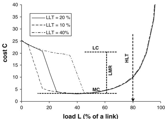
Fig. 1 IP/MPLS layer load-based cost function
