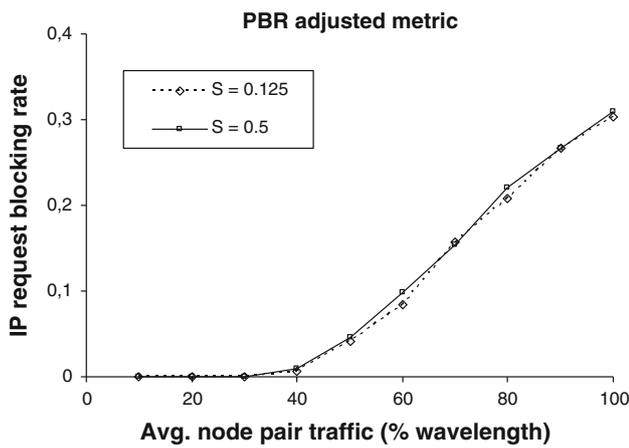
Fig. 5 PBR adjusted hop-count metric; example blocking rates
