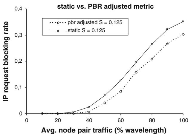
Fig. 6 Static versus PBR adjusted metric for  $S = 0.125$
