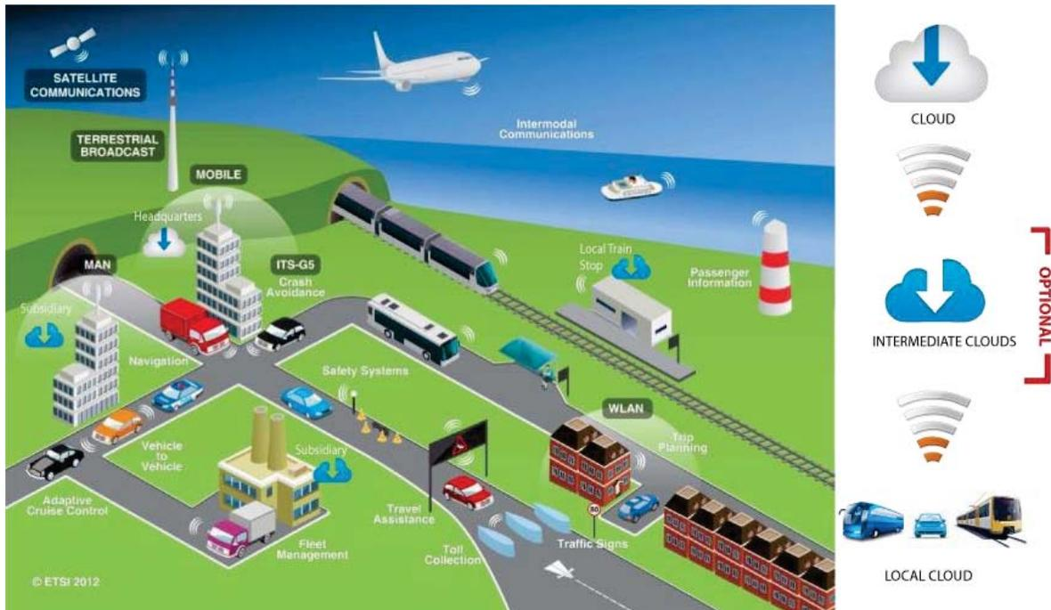
Fig. 1. Hierarchical Cloud Concept for ITS
