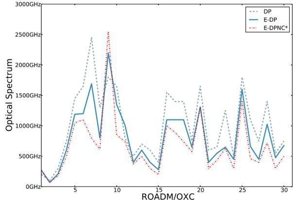
Figure 9. Comparison of the OSP utilization per ROADM/OXC in multiple link failure scenarios.
