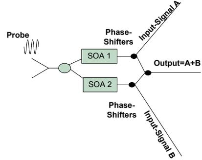
Figure 3. All-optical XOR gate based on Semiconductor Optical Amplifiers (SOA).
